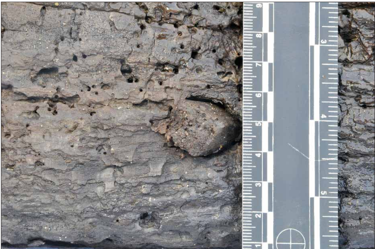
Plate 14: T481 wooden dowel and beetle damage
